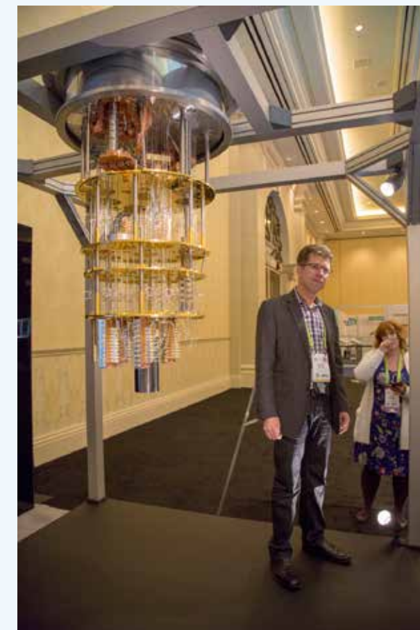
Inside one of the IBM's cryostats wired Quantum System.
