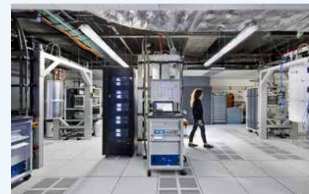
IBM's Quantum Computing Center at the Thomas J. Watson Research Center in Yorktown Heights, New York, holds Quantum Computers in large cryogenic tanks (far right) that are cooled to a fraction of a degree above absolute zero
